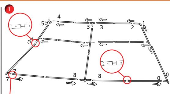
Complete the assembly with the upper horizontal sections to make it easier to fit the internal horizontal support poles.
