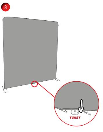
NOTE: Adjustable feet can be used to level frame
