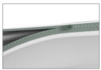
LIGHTS: (OPTIONAL) Place the base of the light fitting in the hole in the middle of the profile. Place both lights on fitting. Run the electric cords inside the print and out the bottom of base.
