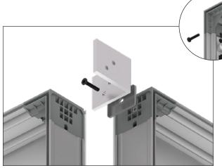
**Step 4:** Complete install of connectors by pushing the DNA Panel into place and instaling screws top and bottom.
