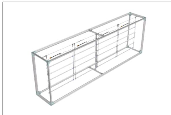
**Step 10:** Attach c-clamps to frame on top and bottom use hex tool. **Place eyelets on top of frame** for use with wiring harness.
