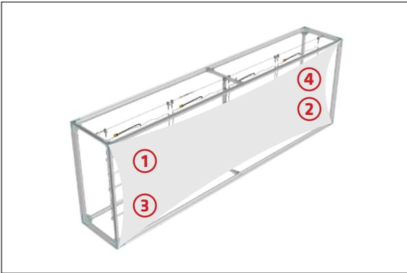
**Step 11:** Fold silicone edge graphics over and install into first corner of frame working outwards 4-6 inches. Repeat on remaining corners starting with the opposite corner. Follow the Graphic Diagram.
