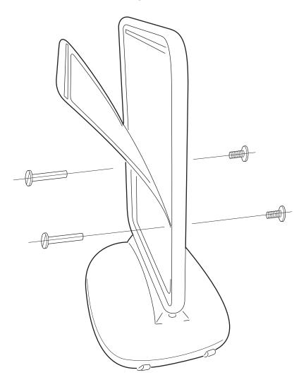
Remove the 2 No. Screws. Remove & discard the damaged panels.
