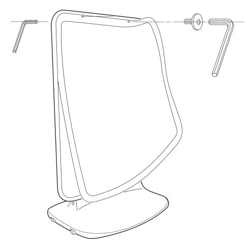
Use the two Allen keys supplied to release one of the fixings. Molegrips may be required to grip the remaining thread to assist in the removal of the second fixing.
