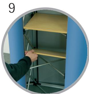
Drop the 3 wooden shelves into position within the structure to complete your Mini Pop Up Counter
