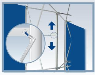
Adjust, with the help of an Allen key, the horizontal stay so that it fits the hole that you have made in the panel. Put the graphic panel back into place.
