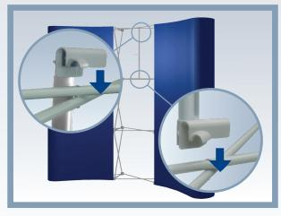
Remove the graphic panel of your choice to get access to the frame. Click firm the upper and lower brackets of the Screen Holder in the cross section of the frame.
