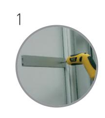
Locate 220mm straight profile in desired position and insert into 8-way post. Secure by tightening expanding clamp grub screw.
