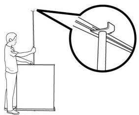
4. Pull up the second graphic and position the end tip of the pole into the profile.
