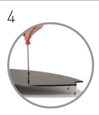
Pre-assemble the two black acrylic shelves to 616mm profiles by aligning the predrilled holes, inserting 4 off countersunk self-tapping screws, and tightening with cross-head screwdriver supplied to secure.
