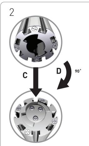
Affix posts (with two brackets) to lower posts by positioning female end centrally over male fitting (C), and rotate until assembly drops into position, continue rotating clockwise through 90° to secure (D). Ensure that all shelf brackets are aligned on one side of the posts (as shown right).
