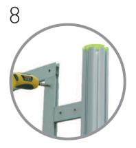
Slot second horizontal rails onto all vertical rails and tighten grub screws.
