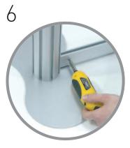
Connect first horizontal rails at the bottom of posts, leaving a 10mm gap between underside of rail and surface of base plate. Tighten clamp screws to secure in place.
