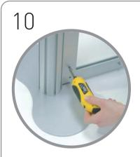
Connect side vertical rails to the bottom horizontal rail. The side vertical rails have one run of tape on them. Strip should be nearest the post when viewed from the front.
