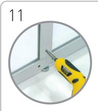
Connect middle rail(s)\* to the bottom rail and tighten grub screws. The middle rails have ta double graphic fitting strip on them. They will balance.
